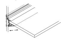
If the shelf board is not level, remove the shelf paying attention not to damage the shelf, and adjust screws at B section to make it level
