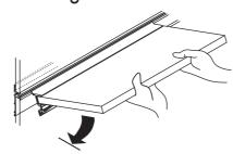
Tilt the shelf board and push the projected area into the slotted panel bracket, then push it downward until the board levels.
