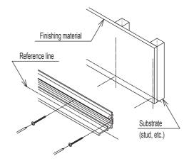
Mark with level, etc. the position to fit the shelf bracket, assuming the height of the horizontal line of the upper surface of the top/bottom bracket as the reference.
