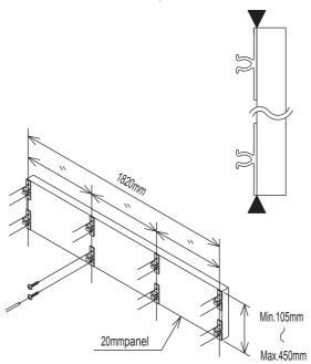
Fit the catches (VT-DF-C20) to the t20 panel prepared by the customer with fixing screws according to the illustration after checking the fitting position. Fit the catches to the necessary number of panels
