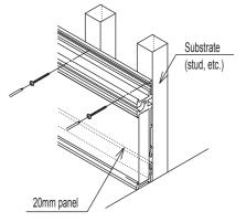
Insert the t20 panel along the bottom bracket
