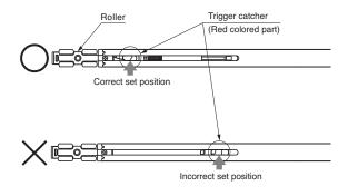
If the position is wrong, pull back the trigger catcher to the correct position using a 6mm diameter round bar.
