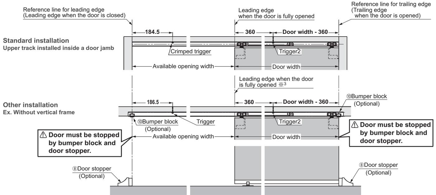
※<sup>3</sup> Determine the trigger position from the leading edge of the door when it is fully opened. If a margin has been set, measure from the leading edge of the door when the door has reached the stopper ⑦.
