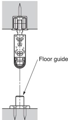
Position the floor guide so that its roller part stays under the door when it is opened or closed.
