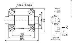
√!\Screws not included Recommended screw and washer M5 hexagon socket head screw × 4 washer 5mm in nominal diameter × 4
