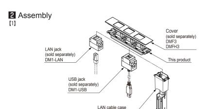
[2] Starting from either end, Hook the jack onto the lip of the bracket and push until a click sound is heard
