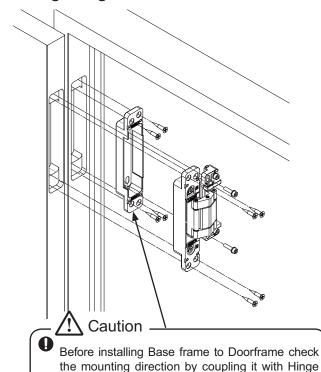
While holding the door, insert Hinge main body into the Base frame on Doorframe. Keep holding the door and fix the hinge with the fixing screws at once.
