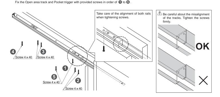
After fixing the track, move rollers and check if there's any misalignment or gap between the track.
