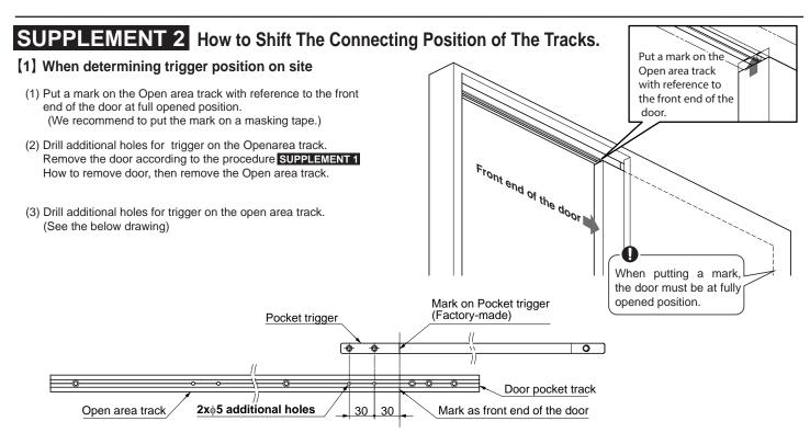
(3)Fixing Open area track Follow the right below figure, since the working sequence is different from regular process.
