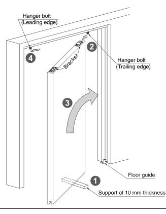
Ensure that hanger bolt head is in straight position as shown for smooth fixation of Holder.
