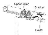
2 Adjust door such that door is parallel to upper track with 8mm clearance between door and floor.
