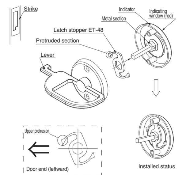
\* In case of left lock type, install parts such that upper protruded section faces door end (leftward).
