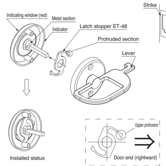
\* For right lock type, set parts such that upper protruded section faces to door end (rightward).
