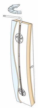
Door straighteners can help prevent doors from bending, due to warpage caused by heat and humidity. Pre-installed straighteners can also correct doors experiencing warpage. Straighteners are designed to be installed at the time of door manufacture, and can be used for swinging doors, sliding doors or lateral opening doors.
